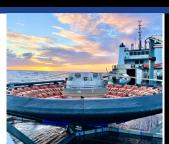
NASA's Low-Earth Flight Test of an Inflatable Decelerator (LOFTID) demonstrated a crosscutting aeroshell — a type of heat shield for atmospheric re-entry.
